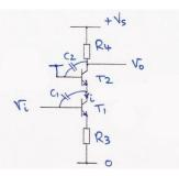
In this circuit the input transistor  $T_1$  has a collector voltage fixed at 3 V - 0.6 V =2.4 V, hence there is no Miller effect with  $C_1$  at the input.
