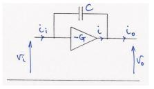
The input capacitance is equivalent to (1+G)C. The magnification of capacitance is known as the Miller Effect. The output capacitance is equivalent to  $\left(1+\frac{1}{C}\right)C\approx C.$
