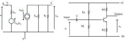
We can ignore  $h_{\rm oe}$  (~ 6%) and  $h_{\rm re}$  (~ 5%) and the small signal model can be sim-
